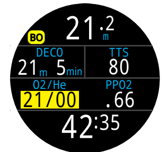
14. Gas Switch Required
